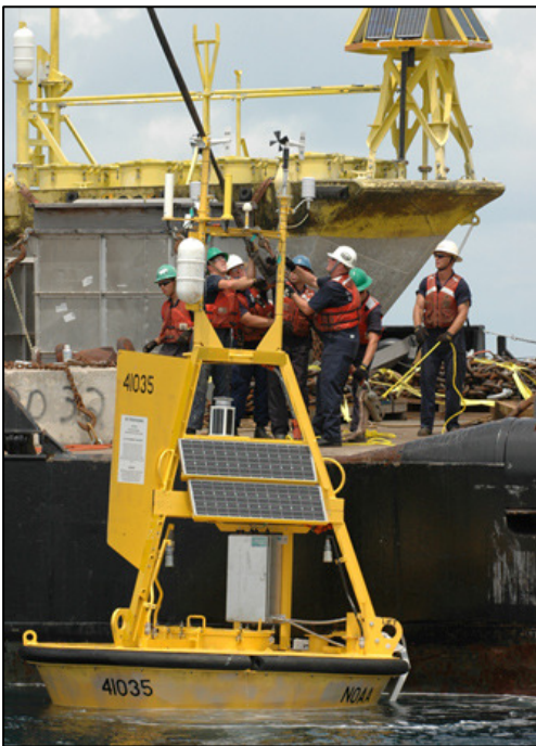
The USCG ELM deploys a UNCW/US Marine Corps weather and oceanographic buoy 5 miles offshore of the Camp Lejeune Marine Corps Base. The buoy provides valuable data for boaters and mariners and plays a significant role in military training and Base operations. Photo: UNCW/Jamie Moncrief
